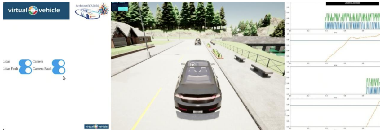
Figure 6: Simulation of the test scenarios in Carla environment simulation in conjunction with the Autoware.AI integration
